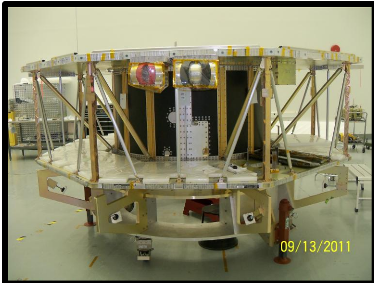
Left: Fit check of MMS FPI sensors on Spacecraft Deck #1
