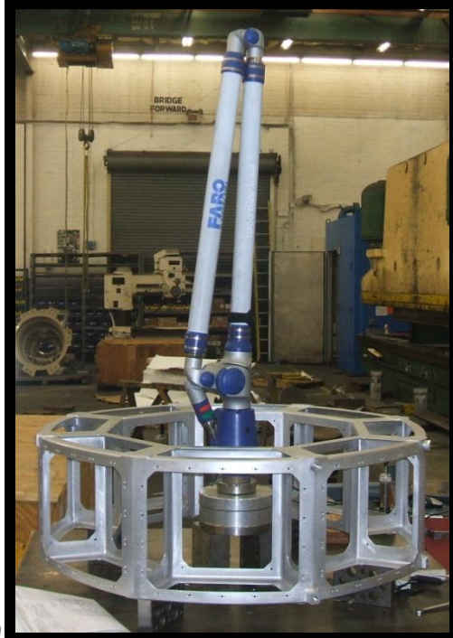
Left: IRIS Final Frame Inspection
